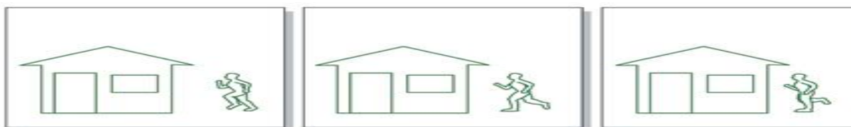
Fig 1. Motion JPEG format, the three images in the above sequence are coded and sent as separate unique images (I-frames) with no dependencies on each other.
